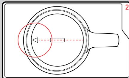
Replace the Lid, ensuring the Lid is aligned correctly with the arrow facing away from the Handle (5) and towards the direction of the Spout (1).
