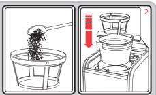
Spoon filter coffee into the Removable Permanent Filter (7). We recommend 7g (approx 1 scoop) of coffee per cup. Place the Filter into the Removable Filter Holder (8) ensuring the Removable Filter Holder aligns into place. The Removable Permanent Filter does not require an additional paper filter. However, you can use a paper filter too, if you choose, but ensure it is suitable for a cupcake shaped filter and matches the dimensions of the Removable Permanent Filter.
