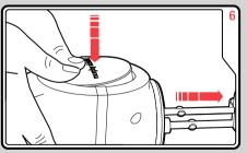
After use switch off at the wall, unplug your Hand Mixer from the mains, and rest the Hand Mixer on its Stand (10). Press on the top edge of the Release Button (5) to remove the Beaters (7), Dough Hooks (8) or Whisk (9) for cleaning.
