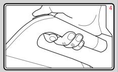
Increase speed gradually using the Vari-Speed Trigger (2). Remove your finger from the Vari-Speed Trigger (2) to switch off.
