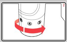
Turn Speed Control Dial (1) to the desired speed.
