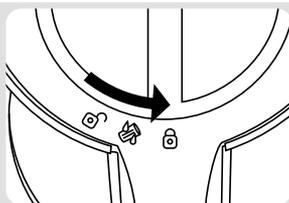
Place the Hopper unit into the Jug ensuring the Lid is locked **5** and in the correct position. Place the Jug onto the Base **2**.
