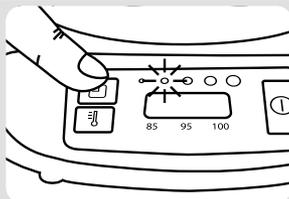
Plug the Tea Maker in. Use the Strength Button **3** to select the desired strength of tea. Press the button repeatedly to cycle through the options.
