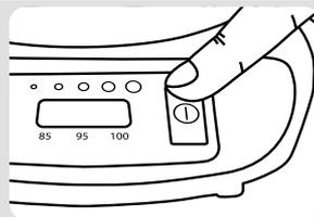
Press the Start Button **15**, the temperature of the water will appear on the Digital Display **11**. When the water has reached the correct temperature, a timer will appear on the screen and countdown until your tea has finished brewing.
